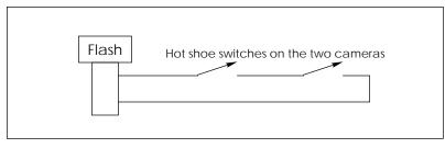
This has the effect of ANDing the two camera hot shoe switches, causing the flash to not fire until both shutters are closed. Kevin cautions: "It was a little tricky getting the wires right, and I got zapped a few times because I forgot that the outer connections of cameras' pc-jacks are already connected via the bodies and aluminum plate they're mounted on".
