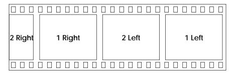
This pattern requires the camera to advance first one frame, then three frames - the extended sequence on film is 1L2L1R2R - 3L4L3R4R - 5L6L5R6R - etc.
